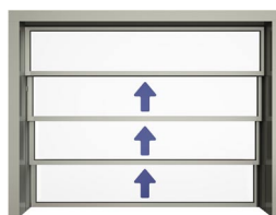
Window with three sliding sections
