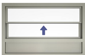
Fixed aluminium section below the window
